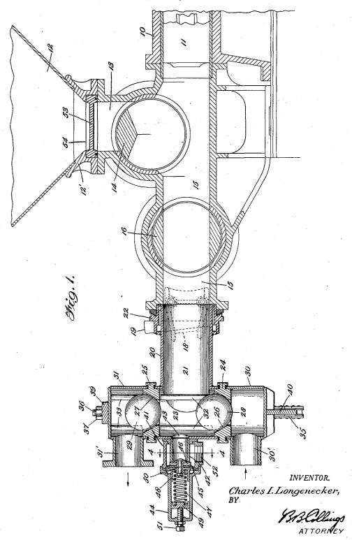
GROUTING ATTACHMENT FOR CONCRETE PUMPS
